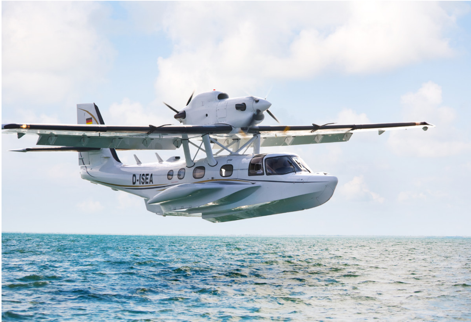
The Seastar's powerful engines sit atop its wings like its predecessor, the Dornier Do X
