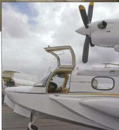
Additional side door for pilot allows easy egress for approaching dockage, beach head and access to engine areas for preflight.
