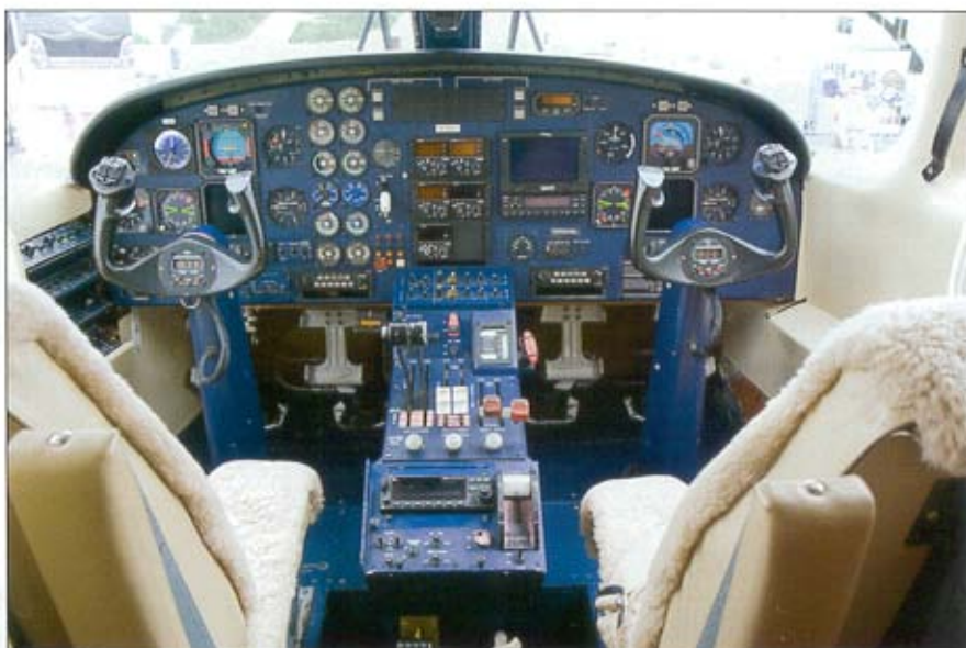
Production aircraft will feature integrated flat panel EFIS/EICAS displays from a yet-to-be-named supplier. Note traditional throttle quadrant as opposed to overhead mounting.
